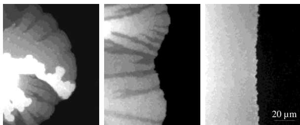
Fig. 6. (a) The kinetic spreading coefficient \beta of DMPC on glass decreases with increasing cholesterol content and exhibits a transition from sliding to rolling. (b) Fluorescence image of the spreading front for 4 mol% cholesterol (sliding regime). (c) Three micrographs as a function of time 7 min, 36 min, 62 min for a DMPC-cholesterol (1:1) membrane on glass. The lipid bilayer fingers on top of the advancing single bilayer slowly fuse into the underlying membrane.
